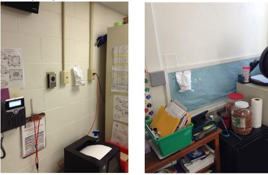
E-PERM® device was deployed inside a breathable Tyvek envelope. Room locations and deployment data are indicated on each envelope.
